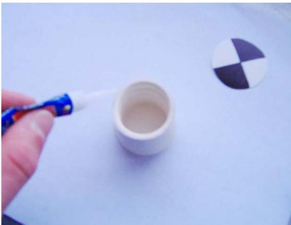
Figure 9: Glue Disk onto Rubber Stopper
