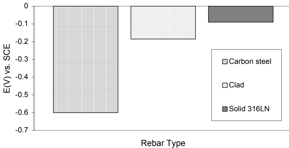
Maximum Open Circuit Potential of Different Rebars in Chloride Contaminated Concrete
