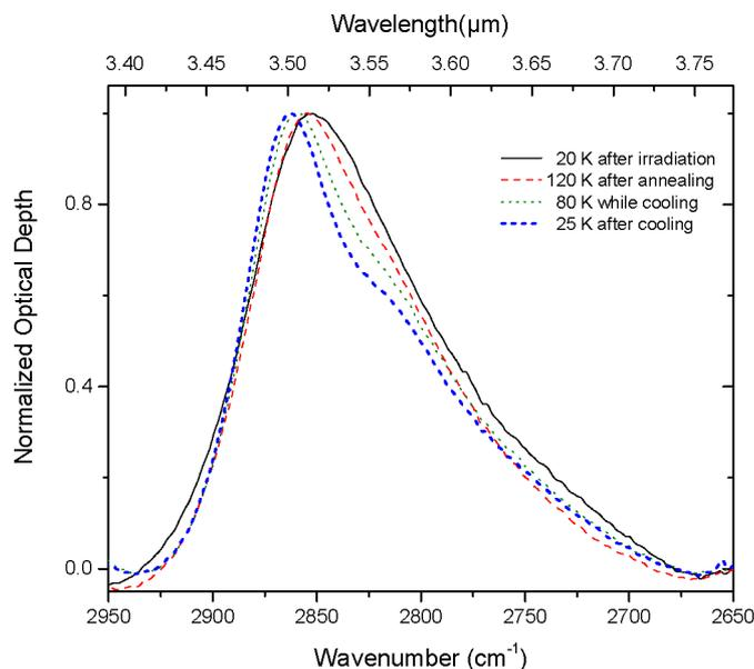
Fig. 8. Changes in the hydrogen peroxide band as the temperature of film is varied for an initially  $5.2 \times 10^{18}\text{ H}_2\text{O}$  molecules  $\text{cm}^{-2}$  water ice film, irradiated with 100 keV  $\text{H}^+$  ions until saturation. The shoulder appearing at short frequencies is only seen at low temperatures after the film has been annealed to 120 K.
