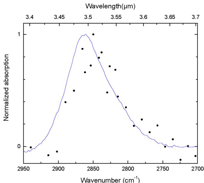
Fig. 9. A comparison of the 3.5- $\mu\text{m}$   $\text{H}_2\text{O}_2$  absorption feature on Europa (circles) and that produced by 100 keV  $\text{H}^+$  ion irradiation of water ice at 80 K (solid line).
