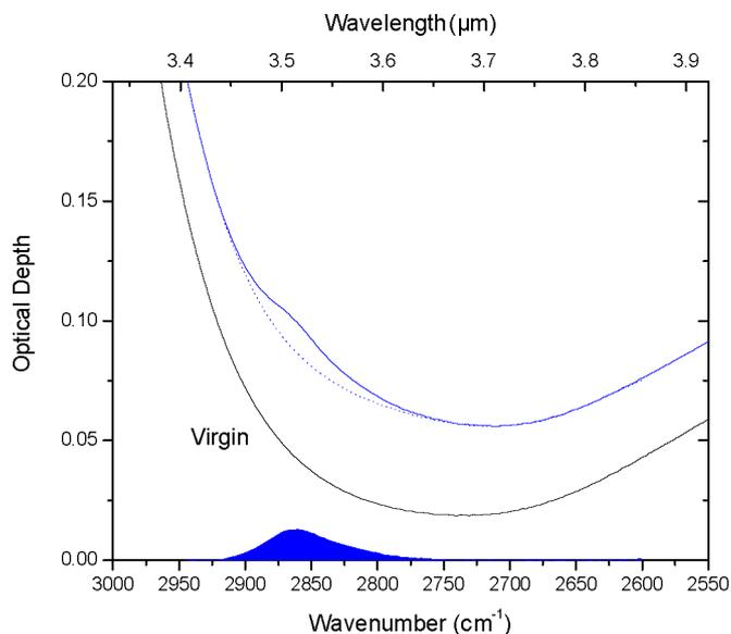
Fig. 2. An example of the baseline fit for the  $\text{H}_2\text{O}_2$  region for the irradiation of  $5.2 \times 10^{18}$   $\text{H}_2\text{O}$  molecules  $\text{cm}^{-2}$  at 80 K with 100 keV  $\text{H}^+$  at a fluence of  $2.7 \times 10^{15}$  ions  $\text{cm}^{-2}$ .
