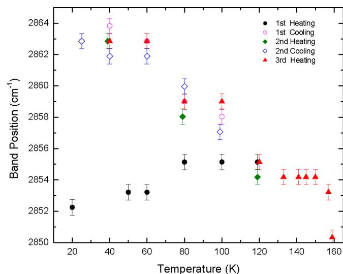
Fig. 7. The peak frequency of the 3.5- $\mu\text{m}$   $\text{H}_2\text{O}_2$  absorption band vs temperature for a water ice film irradiated with 100 keV  $\text{H}^+$  ions at 20 K. For comparison, the position of the band on Europa has been reported to be at  $2857\text{ cm}^{-1}$  (Carlson et al., 1999).
