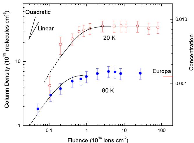
Fig. 3. Fluence dependence of the  $\text{H}_2\text{O}_2$  column density at 20 and 80 K for 100 keV  $\text{H}^+$  irradiation of amorphous water ice. The dotted and solid line together show the fit to the data, using Eq. (15); the dotted part indicates the initial rise. The right axis shows average concentration over the penetration range of the ion, and the average on Europa from Carlson et al. (1999).
