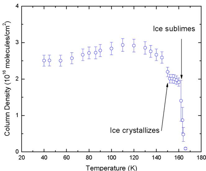
Fig. 5.  $\text{H}_2\text{O}_2$  column density as a function of annealing temperature for a  $2.8 \times 10^{18} \text{ H}_2\text{O molecules cm}^{-2}$  water ice film irradiated by 100 keV  $\text{Ar}^+$  ions at 40 K. The large error bars at the higher temperatures are due to uncertainties in the change of band strength with film thickness as the film evaporates.
