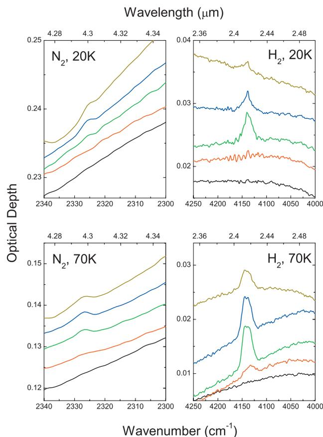
FIG. 2. IR spectra of N<sub>2</sub> (left) and H<sub>2</sub> (right) formed during ion irradiation of a 1:2 ammonia-water mixture irradiated with 100 keV protons at 20 K (bottom) and 70 K (top). Fluences in top panels from top to bottom are: 0, 0.028, 0.38, 2.1, and  $8.3 \times 10^{15}$  ions/cm<sup>2</sup>. Fluences in bottom panels are: 0, 0.11, 1.1, 2.4, and  $9.8 \times 10^{15}$  ions/cm<sup>2</sup>.
