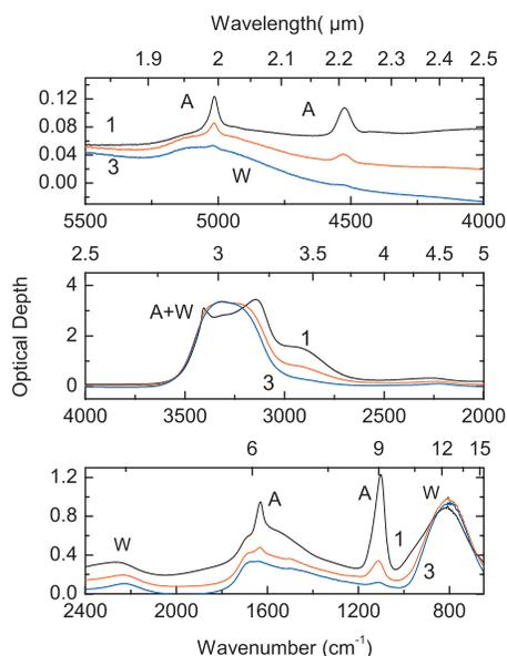
FIG. 1. IR absorption spectra of a 1:2 ammonia-water mixture at 120 K before (1) and after (2)  $1.8 \times 10^{15}$  ions/cm<sup>2</sup> and (3)  $7.1 \times 10^{15}$  ions/cm<sup>2</sup>. We have denoted water as W and ammonia as A.
