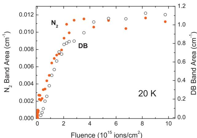
FIG. 5. Fluence dependence of the formation of  $N_2$  (●) and  $DB$  (○) absorptions as indicated by IR spectroscopy in a 1:2 ammonia-water mixture during irradiation with 100 keV  $H^+$  ions at 20 K.
