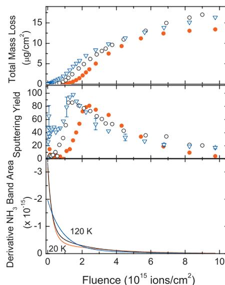
FIG. 6. Total mass loss (top) and sputtering yield (mass loss divided by 28 amu) (middle) and smoothed derivative of the calculated  $NH_3$  BA shown in Fig. 4 (bottom) of a 1:2 ammonia-water mixture during irradiation with 100 keV protons as a function of fluence at 20 K (●), 70 K (○), and 120 K (▽).
