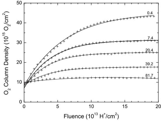
FIG. 6. The column density of  $O_2$  adsorbed during 50 keV proton irradiation at 50 K of 5000 ML thick ice films grown at 70K at an ambient  $O_2$  pressure of  $7.2 \times 10^{-7}$  mbar. The labels of each curve correspond to fluxes in units of  $10^{10}$  ions  $cm^{-2} s^{-1}$ . Lines are fitted with Eq. (8).
