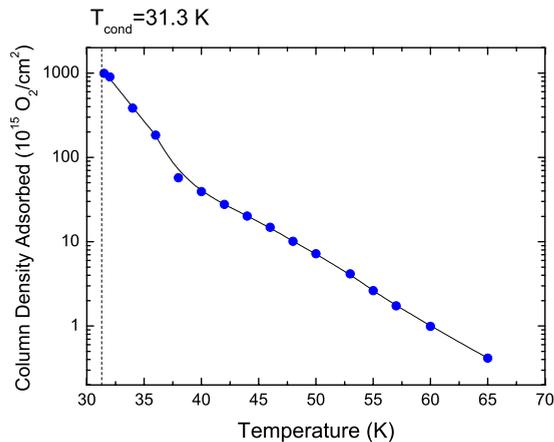
FIG. 4. (Color online)  $O_2$  column density adsorbed on a 5000 ML ice film grown at 70 K and cooled to different temperatures, at a constant  $O_2$  pressure of  $6.6 \times 10^{-7}$  mbar. At temperatures below 31.3 K (dashed line) multilayer condensation occurs at this pressure. The line following the data points is only to guide the eye.
