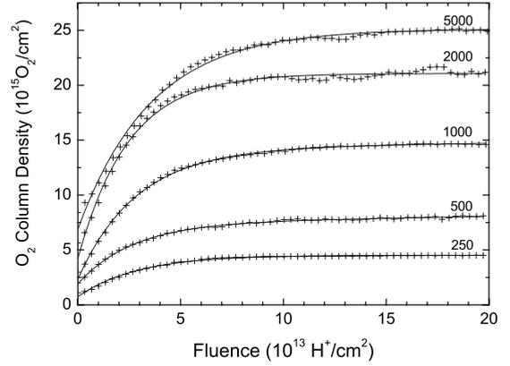
FIG. 8. Fluence dependence of the total  $O_2$  trapped at 50 K for films of different thickness (in units of  $10^{15} H_2O/cm^2$ ) irradiated with a flux of  $2 \times 10^{11}/cm^2 s$  50 keV protons. The crosses are the experimental data and the lines are fits to Eq. (8).
