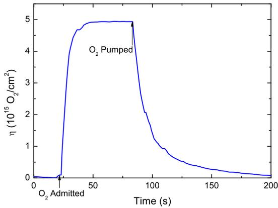
FIG. 1. (Color online) A typical adsorption and desorption curve at 60 K for a 5000 ML ice film grown at 60 K, exposed to an ambient O<sub>2</sub> pressure of  $2 \times 10^{-6}$  mbar.
