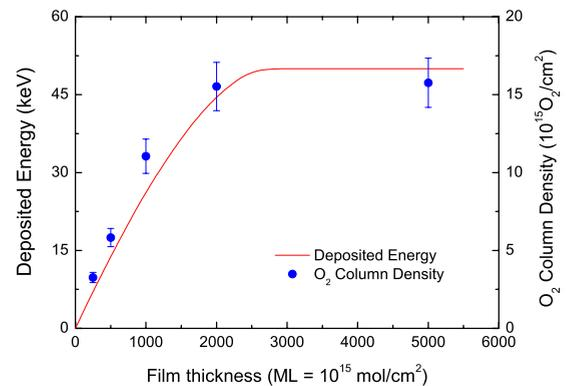
FIG. 9. (Color online) The column density of adsorbed  $O_2$  enhanced by irradiation vs film thickness. The films were grown at 70 K and the irradiations were done at 50 K. The line is the energy deposited by 50 keV protons up to a given thickness, calculated using TRIM.
