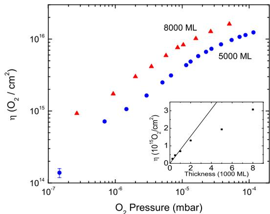
FIG. 2. (Color online) The column-density  $\eta$  of oxygen adsorbed by ice films 5000 and 8000 ML thick (1 ML =  $10^{15}$  molecules/cm<sup>2</sup>). The inset shows the O<sub>2</sub> uptake vs film thickness at an O<sub>2</sub> pressure of  $7.2 \times 10^{-7}$  mbar. Both the growth and absorption temperatures were 60 K.
