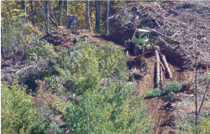
A skid trail is used to move logs and wood products from the stump to the log landing. Source: Virginia Department of Forestry
