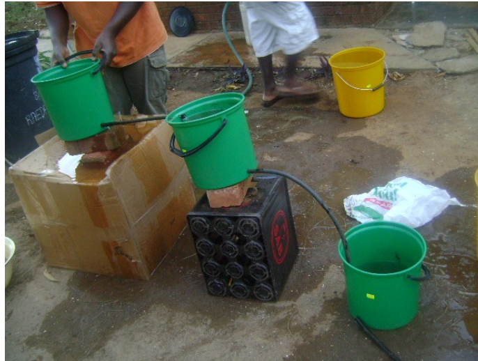
FIGURE 4 AUTHOR TESTING A PROTOTYPE DESIGN WITH AN ADDITIONAL STORAGE TANK BEFORE THE FILTRATION TANK
