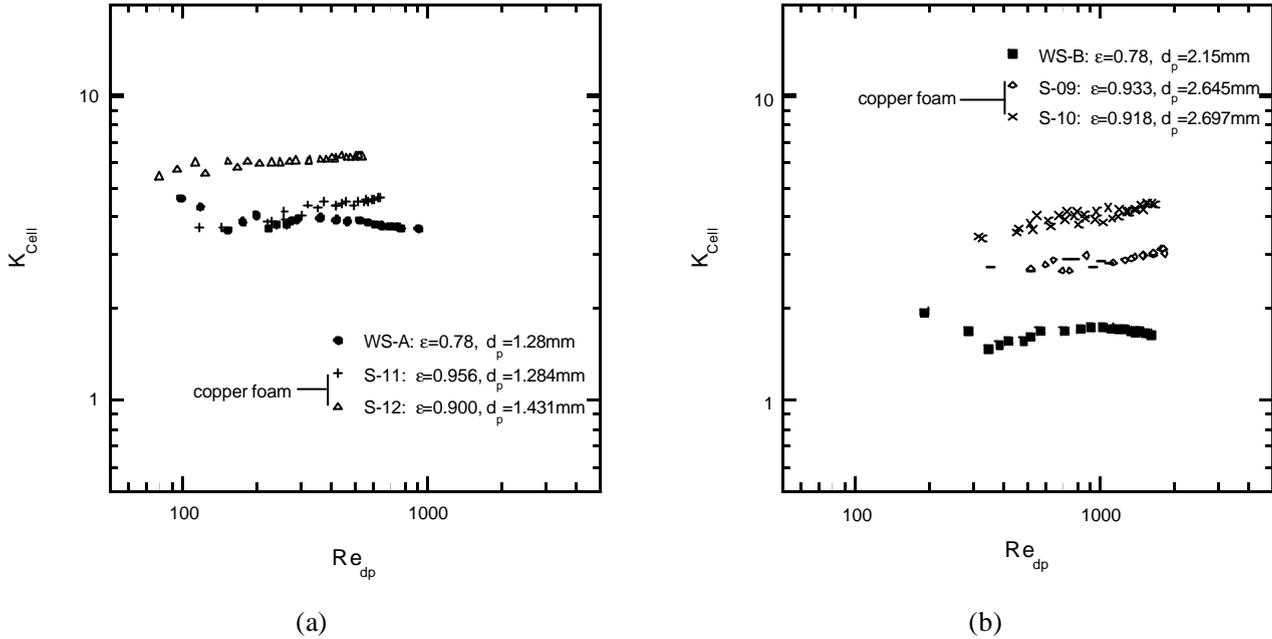
Fig. 5 Comparison of pressure loss coefficient with open-celled copper foams (similar cell sizes) (a) WS-A with copper foam sample S-11 and S-12; (b) WS-B with copper foam sample S-9 and S-10
