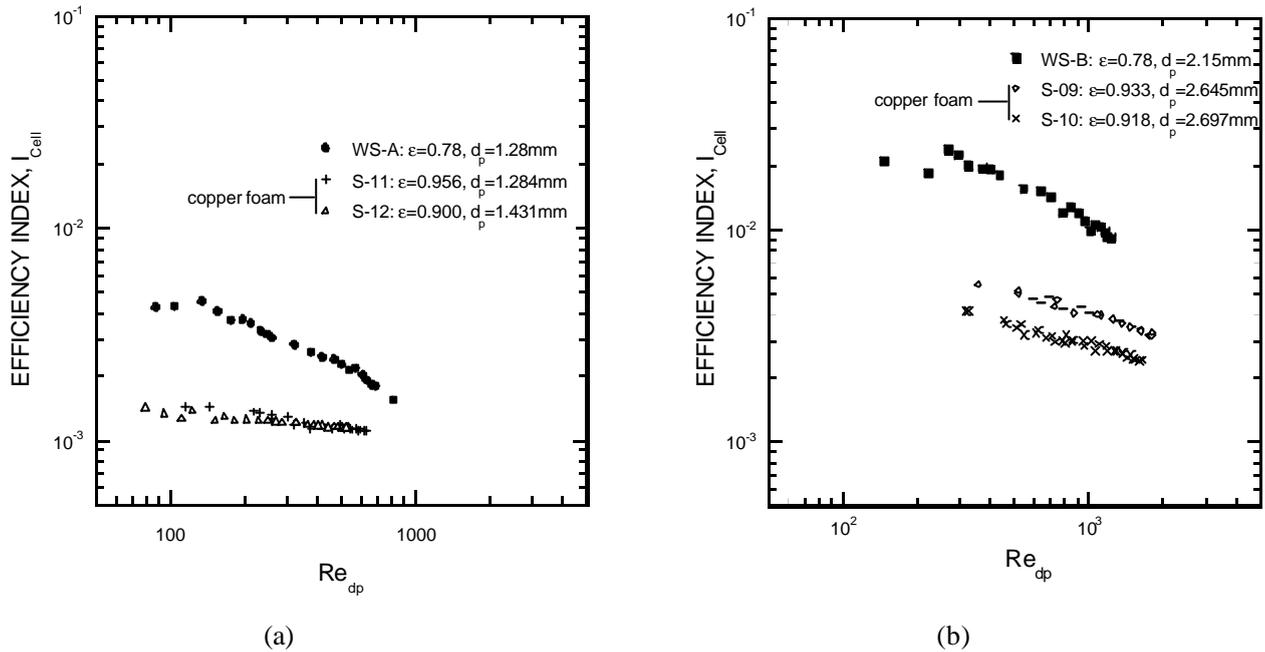
Fig. 9 Comparison of thermal efficiency indices between wire screens and copper foams
