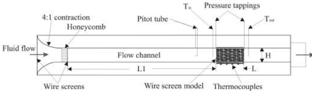
Fig. 3 Forced air convection test rig
