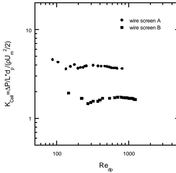
Fig. 4 Pressure loss coefficient as a function of Reynolds number of wire screens
