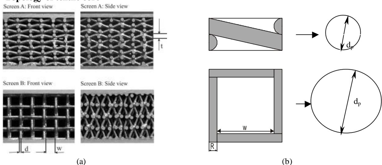
Fig. 2 Textile laminate heat exchangers: (a) images of two different screen meshes; (b) unit cell representation
