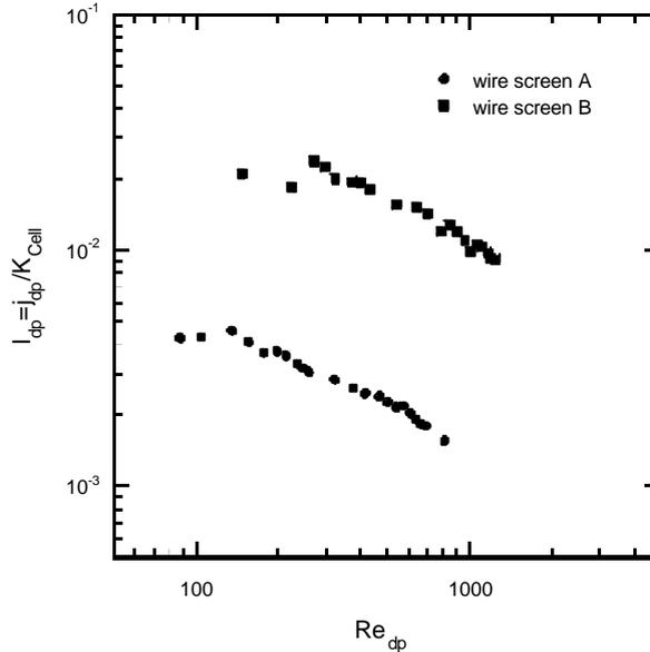
Fig. 8 Thermal efficiency index as a function of Reynolds number
