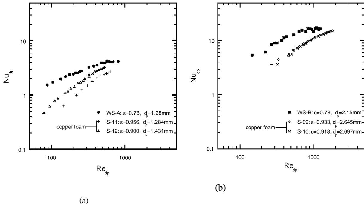
Fig. 7 Comparison of Nusselt number with open-celled copper foams having similar cell sizes
