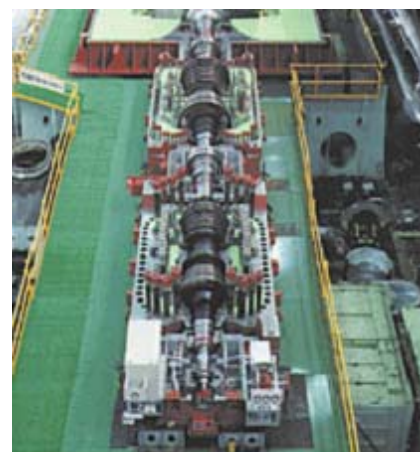
Figure 2: Mitsubishi Heavy Industry Large Turbine Generator
