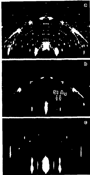
Fig. VIII.5a-c. RHEED patterns taken with a primary energy of E = 15 keV and a direction of incidence of [112] on a Si(111) surface: (a) Clean Si(111) surface with a (7 \times 7) superstructure. (b) After deposition of nominally 1.5 monolayers (ML) of Ag streaks due to the Ag layers are seen on the blurred (7 \times 7) structure. (c) After deposition of 3ML of Ag the texture structure due to the Ag layers develops in place of the (7 \times 7) structure [VIII.3]
